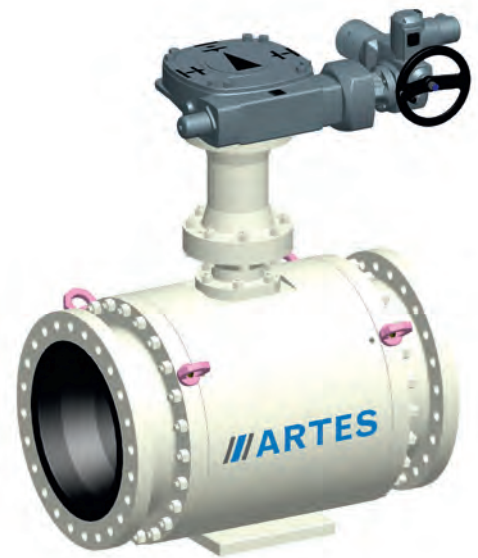
Type 25 with electric part-turn actuator Connections: 1" 900 lbs Location of use: Natural gas drying Medium: Glycol
