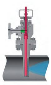
In contrast to other valves that operate according to the lift principle, the ARTES desuperheater utilises rotary movement. The quantity of water to be injected is controlled by the rotation of the valve stem. An additional regulating valve, as is necessary when using unregulated nozzles, is not required here.
