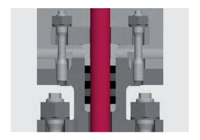
Permanently sealed to the outside: The rotary movement prevents dirt from being pulled into the packing.
