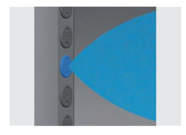
No cross-flow: The leak-tightness between the nozzles is safeguarded by metallic sealing elements. The control over the individual nozzles is adapted depending on the operating conditions. This allows precise control over the injection water quantity in accordance with the specified characteristics curve.
