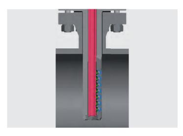
No vibration fractures: Contrary to lift valves, no forces or torques act on the stem after it has been positioned. The flow through the inside of the nozzle stem provides additional protection.
