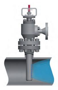
The order in which the nozzles open is determined by the design of the nozzle stem. The nozzles located in the middle of the desuperheater are always the first to inject cooling water.
